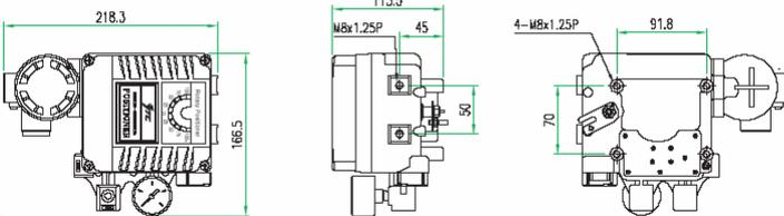
The Electro-Pneumatic Positioner YT-1000R is used for operation of pneumatic rotary valve actuators by means of electrical controller or control systems with an analog output signal of DC 4 to 20mA or split ranges.
