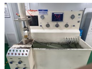
Pressure Test for Large Valve
