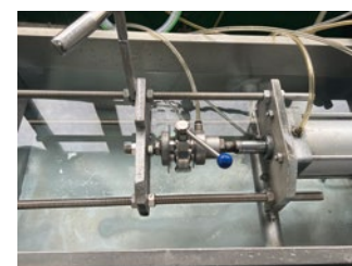
Pressure Test for Small Valve
