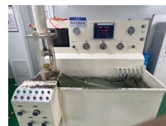
Pressure Test for Large Valve
